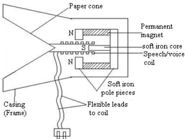
It consists of a light coil of wire known as a speech coil wound tightly round a cylindrical former to which a large thin cardboard cone is rapidly attached. The coil is in a radial magnetic field provided by the permanent magnet which has circular pole.
