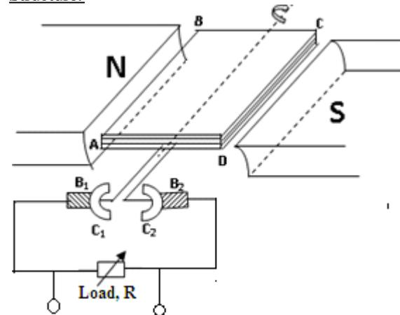
The d.c generator is a device used for producing direct current energy from mechanical energy.
