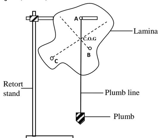
Marking holes: Three holes "A", "B" and "C" are made in the object at the edges far away from each other.
