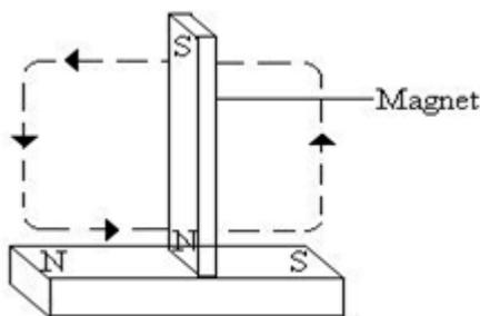
In this method, the steel bar is stroked from end to end several times in one direction with one pole of a permanent magnet.
