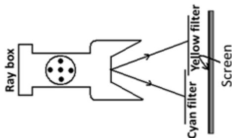
When a yellow filter and cyan filter are placed at some distance from a ray box such that half of their portions overlap.
