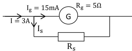
P. d across the shunt = P. d across galvanometer
