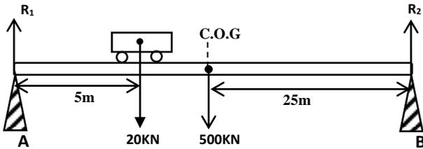
Calculate the reactions at “A” and “B” if the bridge is in equilibrium sum of forces in one direction = sum of forces in opposite direction.
