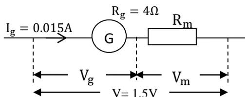
$$V = \left( \text{P. d across the multiplier} \right) + \left( \text{P. d across galvanometer} \right)$$
