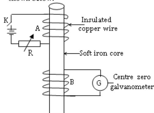
❖ When switch, K is closed, current flows in the primary coil, A and the galvanometer momentarily deflects in one direction and no more deflection there after as the switch remains closed.
