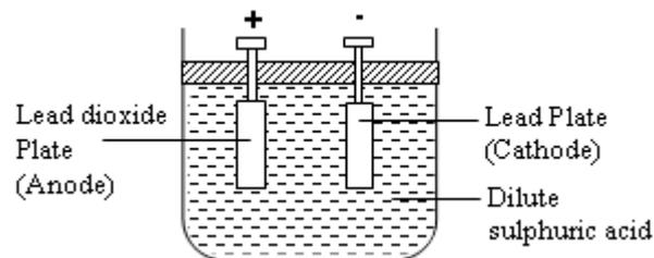
The cathode is lead, the anode is lead dioxide and the electrolyte is dilute sulphuric acid.
