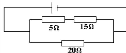
First determine the effective resistance,  $R_s$  for the resistors in series.
