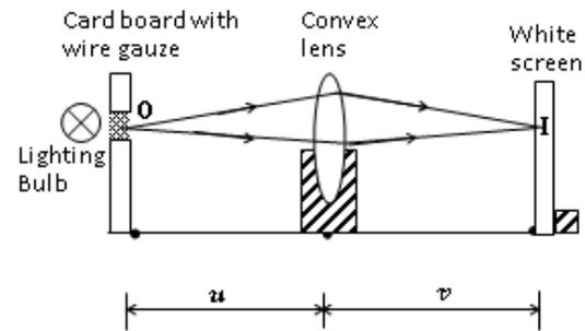
Using an illuminated object, O at a measured distance,  $u$ , move the screen towards and away from the lens until a clear image of the cross wires is obtained on the screen.
