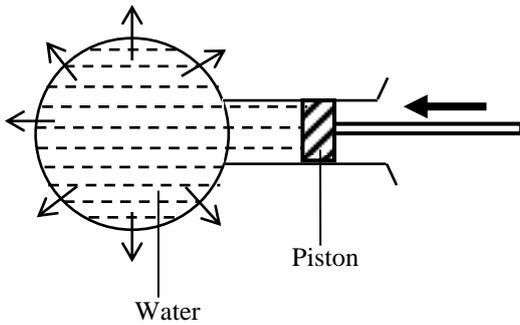
Holes of equal size are drilled in a round bottomed flask and covered with cork. The flask is then filled with water and the piston pushed inside the flask. Water shoots out equally in all directions, and travels equal distances. This verifies Pascal's principle.
