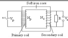
This is stationed near the consumers and in electrical appliances. It changes the output voltage to a lower value. The number of turns in the secondary coil is less than those in the primary coil.
