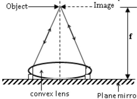
The distance from the pin O to the lens is thus measured and it is equal to the focal length,  $f$ , of the lens.
