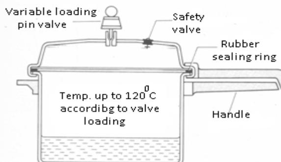
Cooking with a pressure cooker is faster than ordinary cooking because most of its top surface is covered leaving just a small opening to let out vapour.
