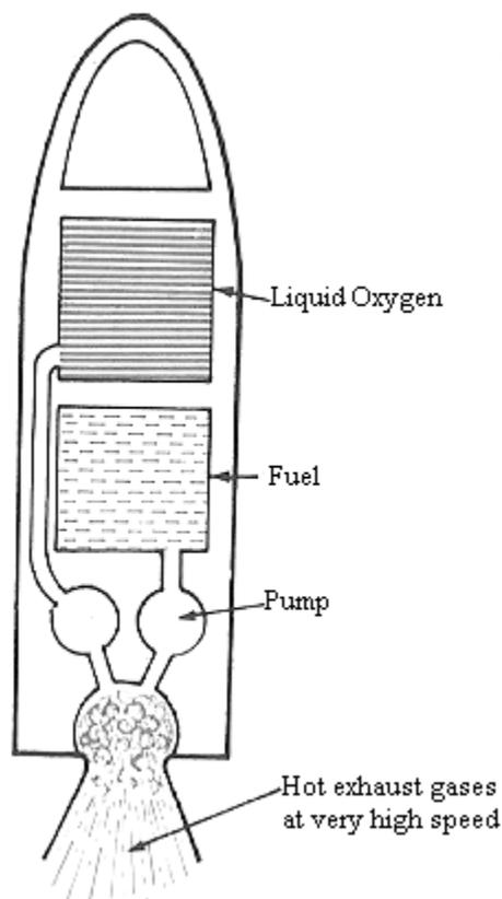
**Principle:** the jet and rocket engines work on the principle that momentum is conserved in explosion.
