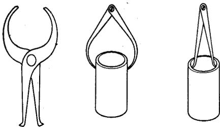
The distance between the jaws is after wards measured on an ordinary scale like a metre-rule.
