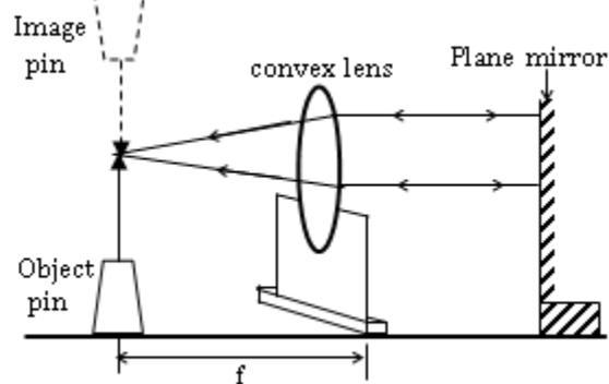
**NOTE:** Rays from O passing through the lens are reflected from the plane mirror M and then pass through the lens a gain to form an image. When O and I coincides the rays from O incident on the mirror must have returned a long their incident path after reflection from the mirror. This happens if the rays are incident normally on the plane mirror, M. The rays entering the lens after reflection are parallel and hence the point at which they converge must be the principle focus.
