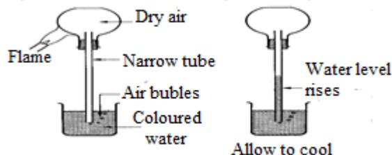
In the above set up the flask is slightly heated. Air bubbles will be seen coming out from the other end of the tube
