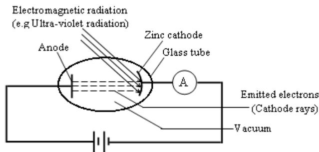
Electromagnetic radiations (eg Ultra violet radiation) are directed onto the cathode and supplies sufficient energy that causes the liberation of electrons.
