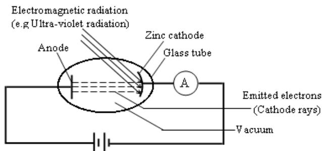
When the cathode was irradiated with ultra violet radiation, the ammeter gave a reading
