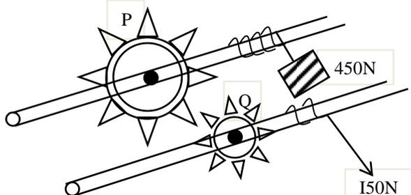
Two gear wheels P and Q with 80 and 20 teeth respectively, lock each other. They are fastened on axles of equal diameters such that a weight of 150 N attached to a string wound around one-axle raises a load of 450N attached to a string wound around the other axle. Calculate the;
