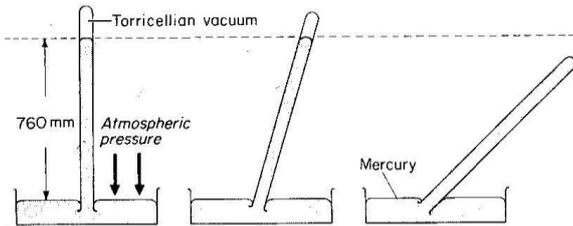
When the tube is tilted as in the diagram, the vertical height of column “h” of mercury remains the same but the length of mercury increases.
