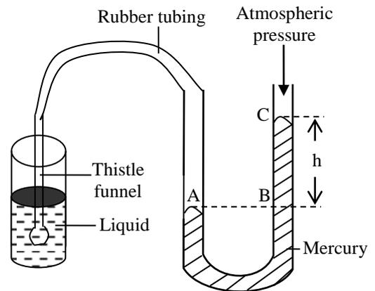
One arm of the manometer is connected to a thistle funnel whose base is covered with a thin membrane and the other end remains open to the atmosphere.
