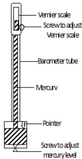
It is constructed like a simple mercury barometer but with a provision for accurate determination of atmospheric pressure.
