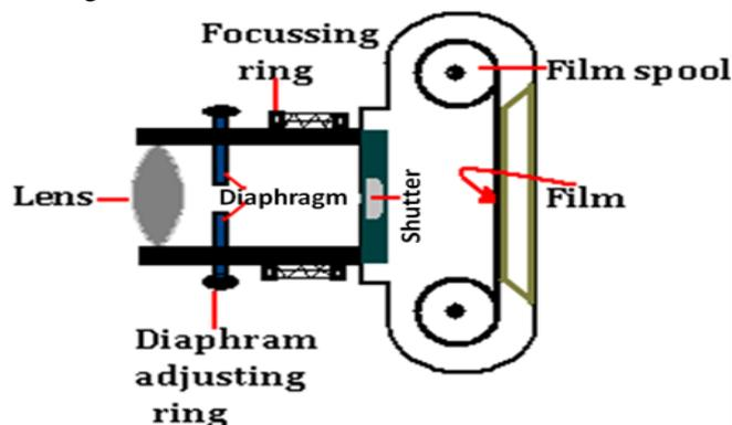
The film contains chemicals that change on exposure to light. It is developed to give a negative. From the negative the photograph is printed.
