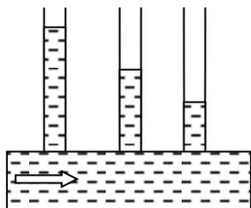
When the liquid flows through the uniform tube, the level goes on decreasing as shown in the diagram, the faster the liquid, the lower the pressure.
