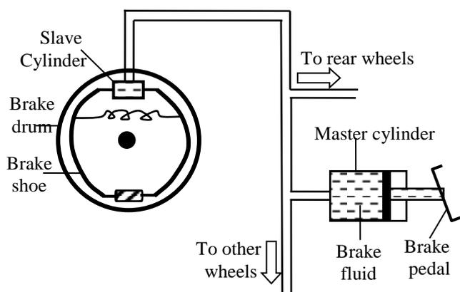
When the brake pedal is placed, the pressure exerted inside the master cylinder is transmitted equally to all the slave cylinders.
