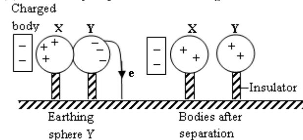
To charge the two spheres simultaneously such that they acquire the same charge, Sphere Y (one remote to the
