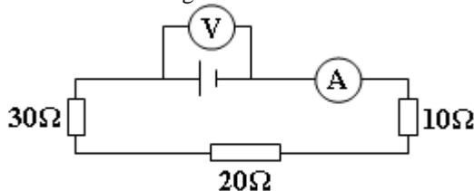
Let  $R_1=10\Omega$ ,  $R_2=20\Omega$ ,  $R_3=30\Omega$ ,  $I=0.2A$ ,  $V=?$
