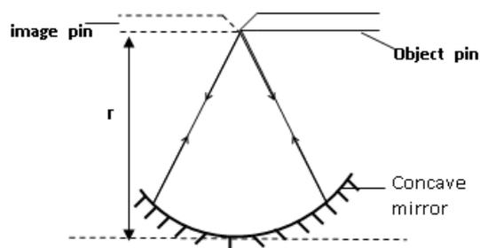
A concave mirror is placed horizontally on a bench. An optical pin is clamped horizontally on a retort stand so that the tip lies along the principal axis of the mirror.
