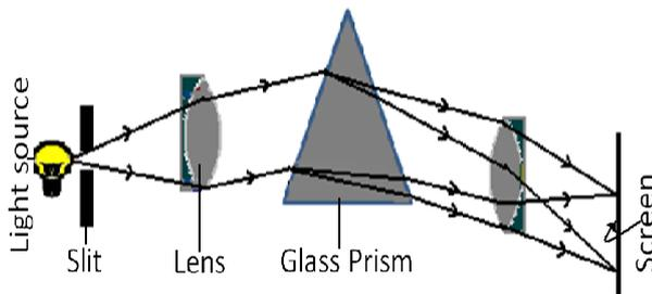
An illuminated slit is placed at the principle focus of a converging lens so that a parallel beam of white light emerges and falls on the prism.
