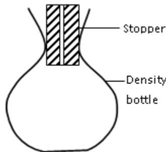
The bottle contains exactly the same volume when the liquid level is at the hole.
