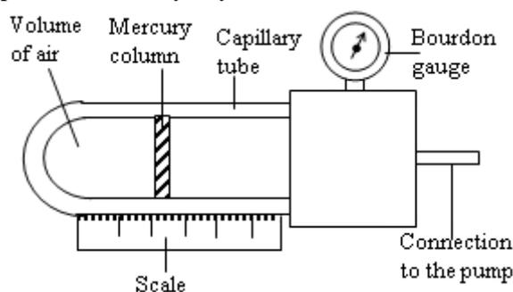
Trap dry air in the capillary tube using the mercury column.
