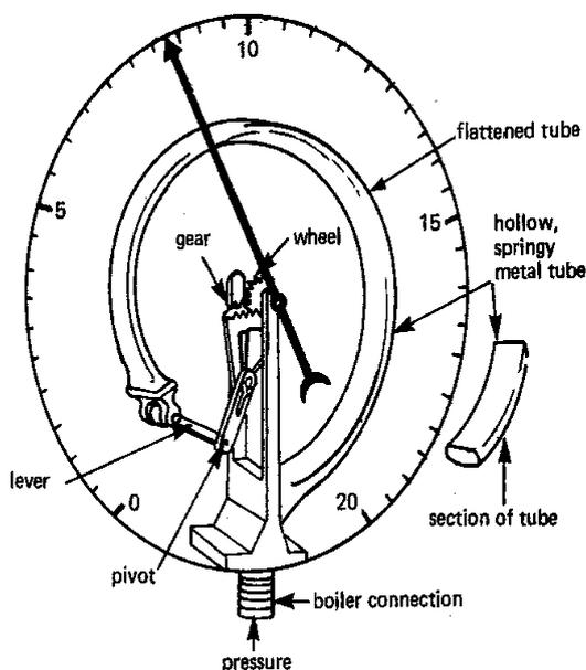
Bourdon gauges are commonly used at filling stations.
