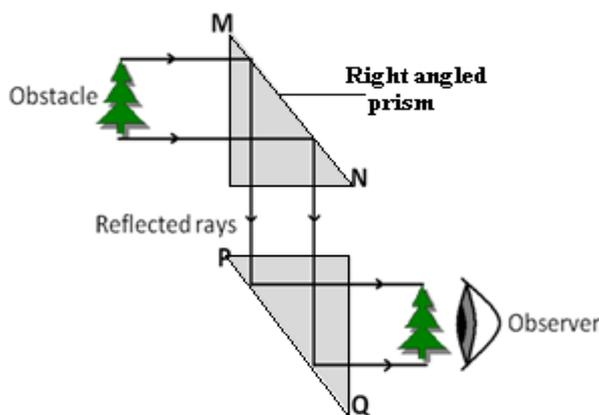
Light from a distant object meets the surface MN at  $45^\circ$ ; so light is totally internally reflected downwards.
