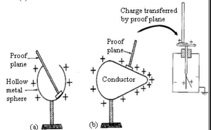
When the proof plane is placed on the outside surface of a charged hollow conductor, charge is transferred to the uncharged G.L.E, the leaf diverges as shown in (a). This proves that charge was present on the outside of the surface.
