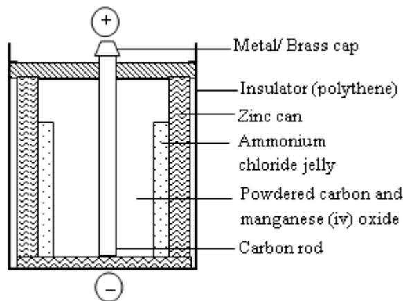
Carbon is the anode and Zinc is the cathode. The electrolyte is ammonium chloride jelly. The chemical reaction between zinc and ammonium chloride is the source of electrical energy in a dry cell and therefore e.m.f is up.
