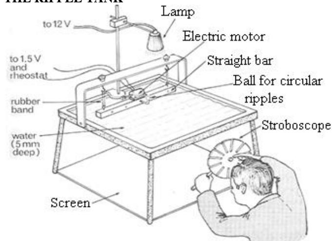
A ripple tank is an instrument used to study water wave properties. It is a shallow glass trough which is transparent. The images of the wave are projected on the screen which is placed below it.
