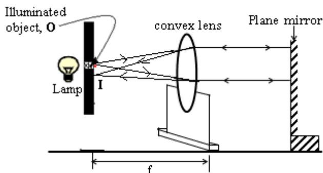
The position of the lens holder is adjusted until a sharp image of the object is formed on the screen alongside the object itself. The object will now be situated at the focal
