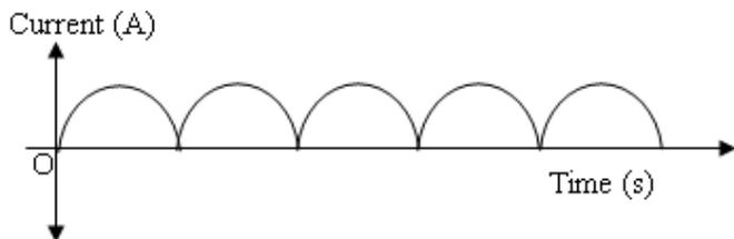
A moving coil galvanometer can be used to measure the average value of the current,  $\langle I \rangle$ .
