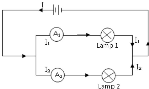
Ammeters are for measuring the current in a parallel circuit. It's characteristic in parallel connections to derive current whenever it reaches the parallel arms of the circuit. But current later recombines to form the original current again before it returns to the cell.
