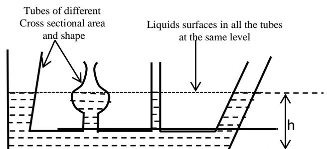
A liquid is poured into the communicating tubes of different cross-sectional areas.
