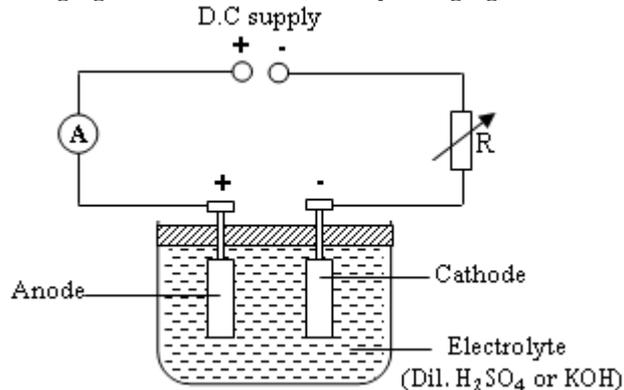
An accumulator is recharged by passing a current through it from a D.C supply in the opposite direction to the current it supplies.
