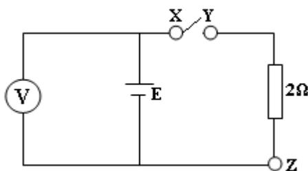
The voltmeter reads 1.5V when the switch is open.
