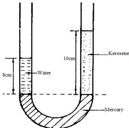
Pressure of kerosene = Pressure of water (since both tube are open to the atmosphere)
