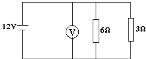
Calculate the current through the resistors.
