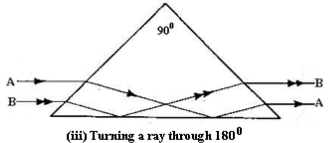
The critical angle of glass is  $42^\circ$  and rays are incident normally on face PR. At face PQ, the rays are incident at  $45^\circ$  so total internal reflection occurs.
