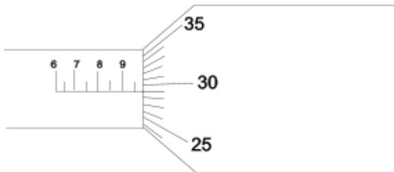
Sleeve scale reading = 9.5 mm
