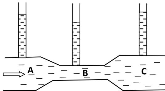
The pressure falls in the narrow part B but rises again in the wider part C. This is because, since B is narrow, the speed at which the liquid moves through it is higher, hence the fall in pressure.
