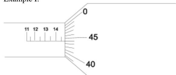
Sleeve scale reading = 14.50mm
