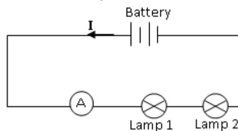
Which is a series connection and current being measured in series.
