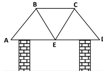
In order to determine each of the girders whether its a tie or a strut, each of the girders is removed and the effect is noted.
