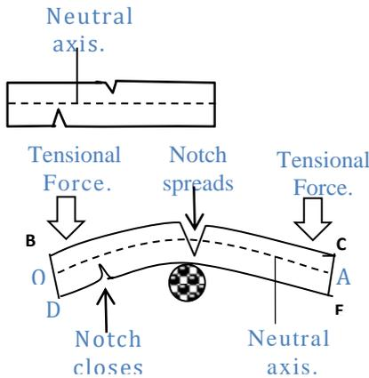
Glass tubes are easily broken after notch is made on the side.
