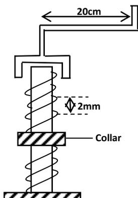
If the car bears down on the car with a force of 5000N and that efficiency of a screw jack is 15%. Calculate the;
