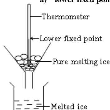
i) Placing thermometer in ice
