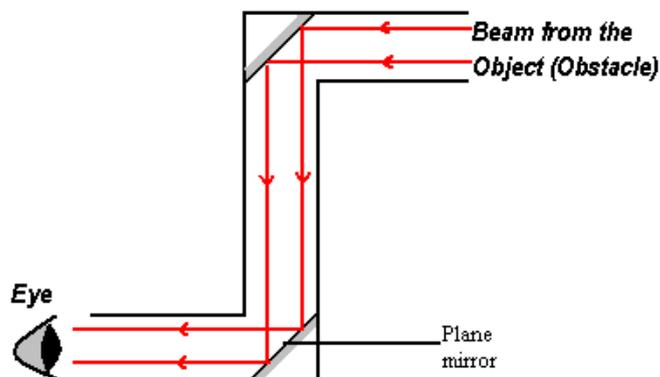
The arrangement has two plane mirrors facing each others and fixed at  $45^\circ$ . Light from a distant object is turned through  $90^\circ$  at each reflection.
