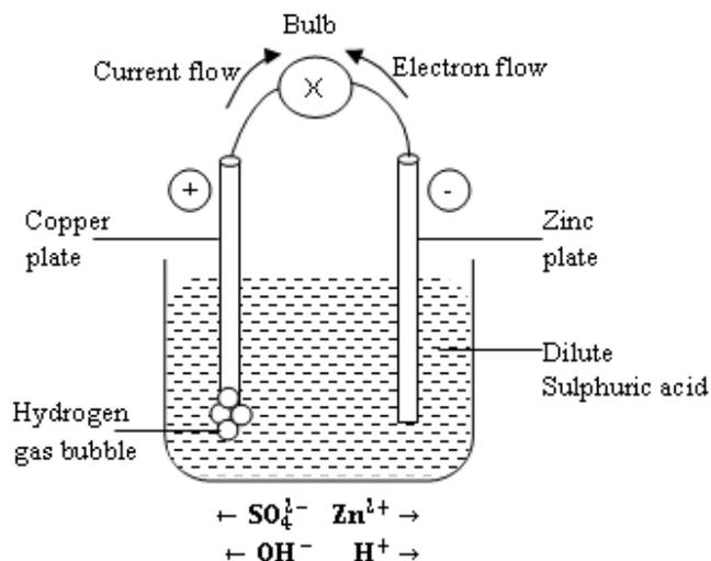
**Mechanism of the simple cells**
