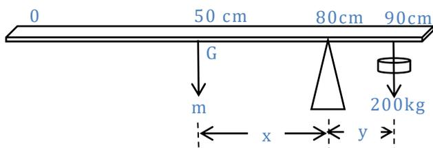
**Example 4:** A uniform beam 2m long is suspended as shown below. Calculate the mass of the metre. (Ans: m=16kg)
