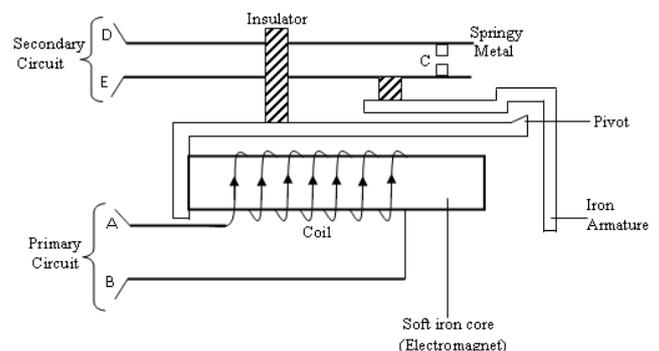
When current flows in the coil from the primary circuit AB, the soft iron core is magnetized and hence attracts the L-shaped iron armature.
