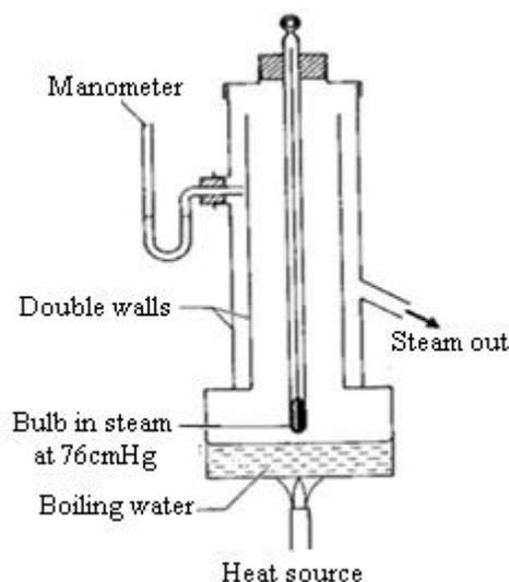
(i). Placing thermometer in steam
