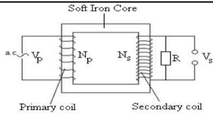
This is usually installed in power stations and transmission stations. It changes the voltage to a higher value by using more turns in the secondary coil than in the primary to the ratio of the output voltage required
