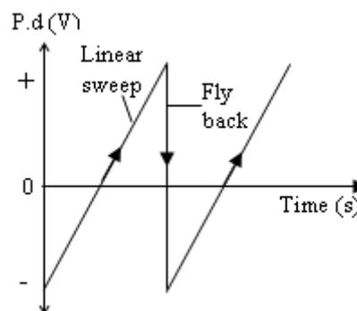
**Note:** During the fly back, the control grid is automatically made more negative thereby suppressing the brightness of the spot.
