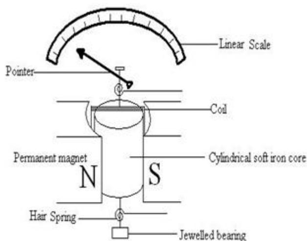
It consists of a rectangular coil with many insulated turns wound on an aluminum former, soft iron cylindrical core between the curved poles of a powerful permanent magnet, the springs which control the rotation of the coil, a pointer and a linear scale. The current is led in and out by two hair springs.
