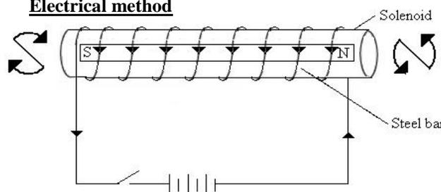
The material to be magnetized is inserted into a solenoid to which a steady d.c is connected to flow.
