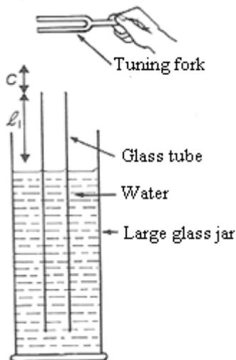
$C =$  End correction,  $l_1, l_2 =$  Length of air columns.
