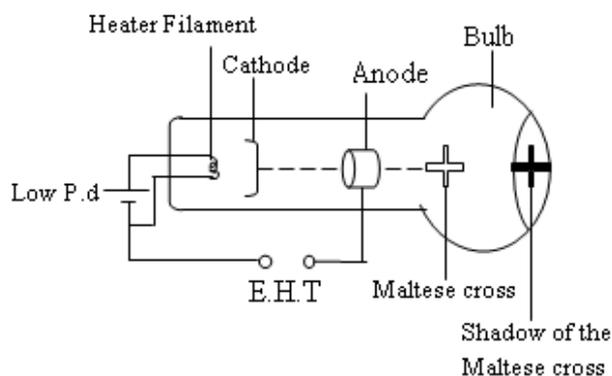
Cathode rays are incident towards the Maltese cross. A shadow of the cross is formed on the fluorescent screen. The formation of the shadow verifies that cathode rays travel in a straight line.
