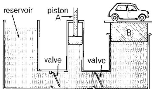
This is commonly used in garages; it lifts cars so that repairs and service on them can be done easily underneath the car.
