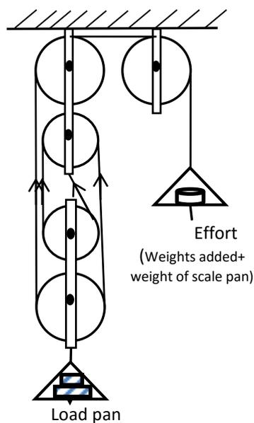
**Determining effort:** A known load is placed on the load pan and known weights are added to the effort pan until the load just rises steadily when given a gentle push.
