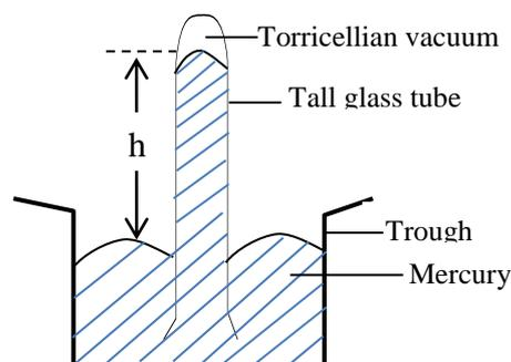
From the above apparatus, when the air above the mercury in the bottle is pumped out, the column falls.
