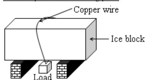
When pressure is increased by the weighted copper wire
