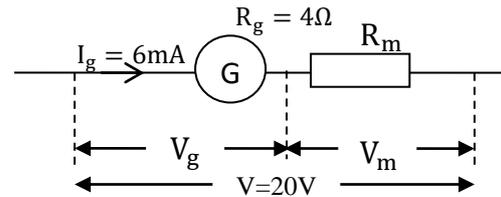
$V = (\text{P. d across the multiplier}) + (\text{P. d across galvanometer})$
