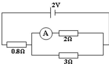
Find the reading of the ammeter, A.
