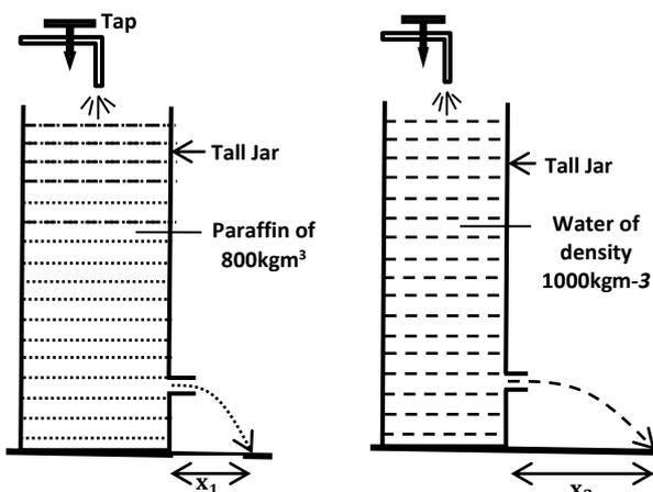
Two tall jars of the same size and height, each with a hole punched at equal depth are used.
