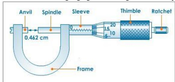
For each turn the spindle moves through 0.5mm. The fraction of each turn is indicated on the thimble. This has a scale of 50 divisions on the thimble and represents  $\frac{1}{50}$  of half a millimeter i.e.  $\frac{1}{10} \times 0.5$  mm = 0.01mm.
