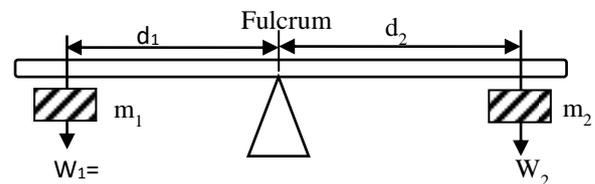
The metre rule is balanced horizontally on a knife-edge and its centre of gravity, G noted.
