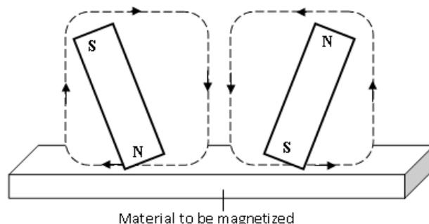
In this method, the steel bar is stroked several times from the centre outwards with unlike poles of the two permanent magnets.
