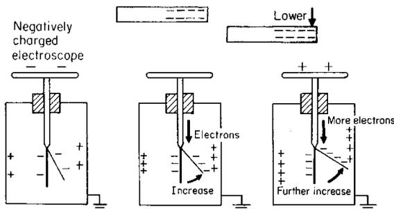
Bring the body under test near the cap of a **charged G.L.E.**
