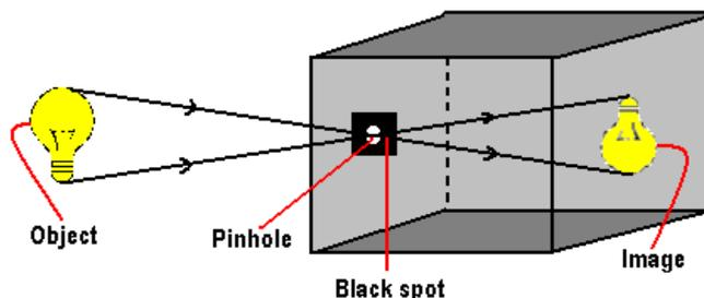
Pin hole camera consists of a closed box with a small hole(pin hole) on face and a screen of tracing paper on the opposite face.
